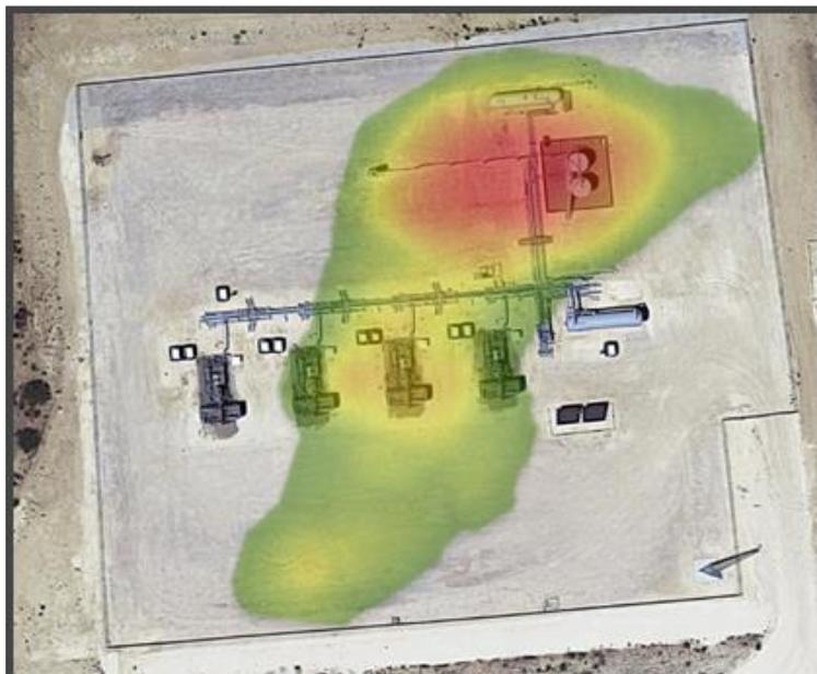
*Fig. 9 Post-flight high-resolution methane concentration heat map.*
